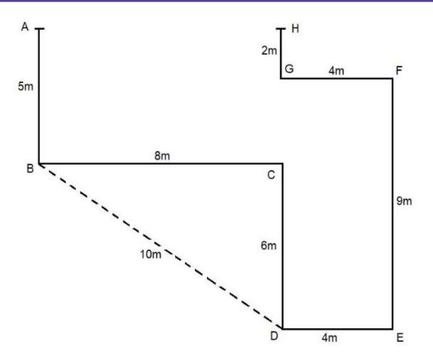
The shortest distance between point B and point D =  $\sqrt{8^2 + 6^2}$  =  $\sqrt{64 + 36}$  =  $\sqrt{100}$  = 10m
